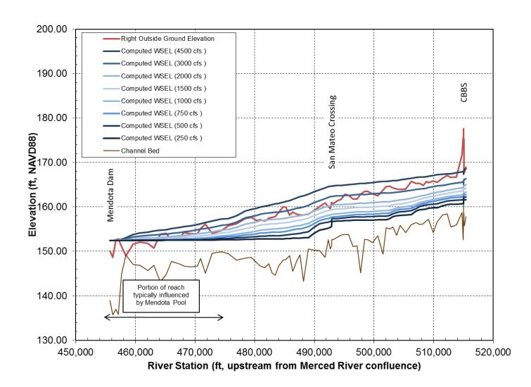
Figure 7. Comparison of outside ground elevation with computed water-surface elevations along right levee in Reach 2B.
